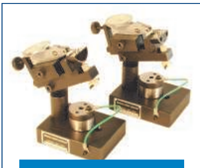
This pair of gages uses test indicators. The delicate tips are guarded, and each station pivots for easy part loading.
