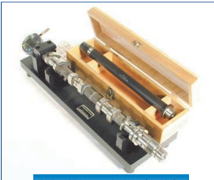
Checks width between shoulders of camshaft
