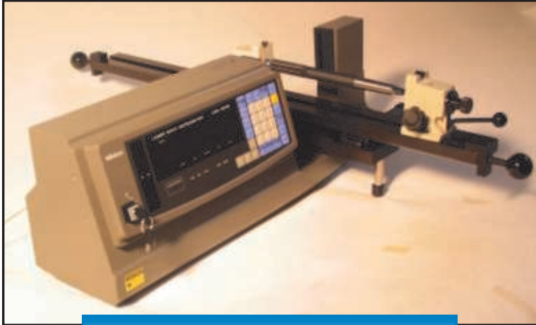
Checks reamer OD using laser scan micrometer
