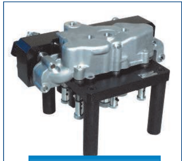
Checks 18 hole positions on mating part
