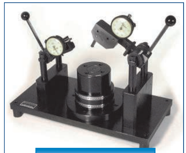
Custom Ball Arbor Checks Runout
