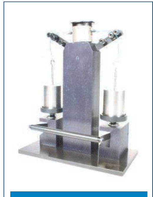
Checks tensile strength using precision weights and spring loaded release handle to eliminate shock load
