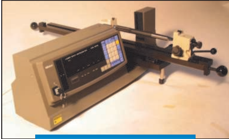
Checks reamer OD using laser scan micrometer
